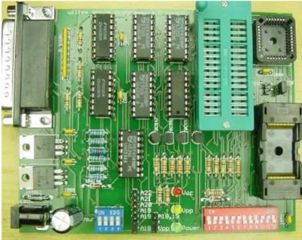
Board 4.5 has no SF erase option and no support for serial eeproms and Microchip PIC's.
